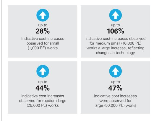
The costs above represent replacement capex investments for replacement treatment works, constructed using typical industry costing approaches. The sample data used, however, is from a less efficient wastewater company, and therefore may represent inefficient (worst case) costs.
