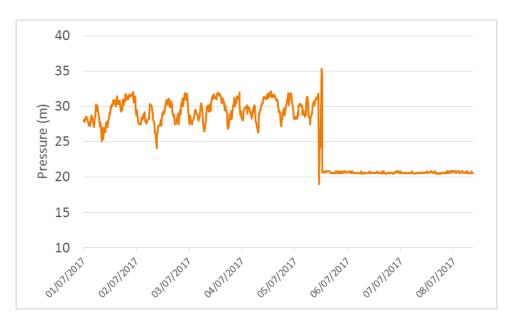
Figure 43 Pressure before and after optimisation
