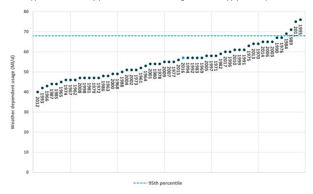
Figure 38 Modelled weather dependent usage for each year<sup>76</sup> with a full set of available weather data
