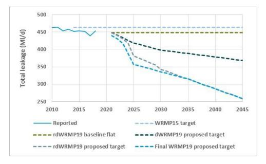
Figure 35 Reported total leakage and our Final WRMP19 proposed target (incorporating a 20% leakage reduction in AMP7), against our WRMP15 target (sometimes referred to as our "current commitment"), a flat target from the Final WRMP19 baseline<sup>70</sup> and our Draft and Revised Draft WRMP19 proposed targets
