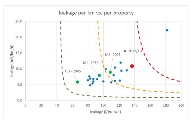
Figure 33 Industry comparison leakage per km vs. leakage per property<sup>66</sup>
