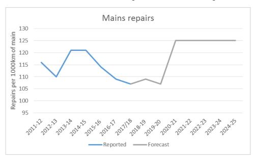
Figure 49 Number of mains repairs per 1000km of main
