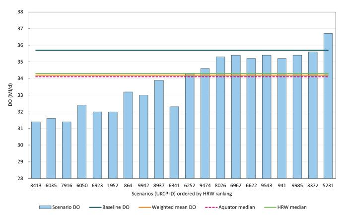
Figure 8 Graph of Carlisle Resource Zone UKCP09 Aquator™ deployable output results for the 2080s, ordered by the drought index ranking
