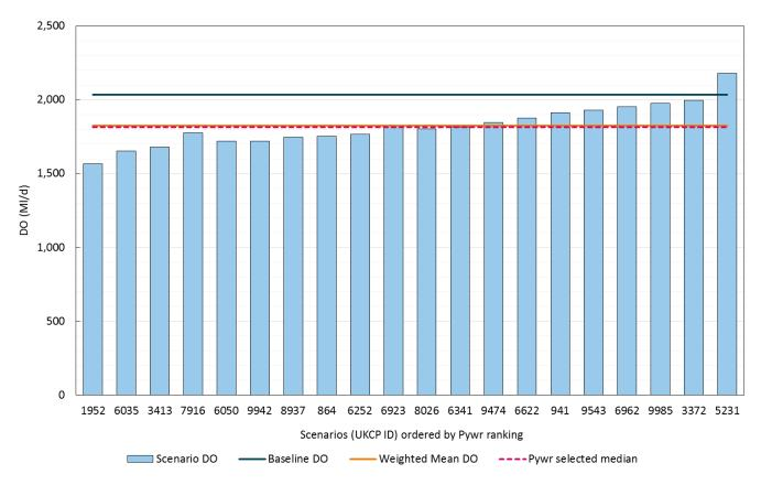
Figure 7 Graph of Strategic Resource Zone UKCP09 Aquator™ deployable output results for the 2080s, ordered by the Pywr ranking
