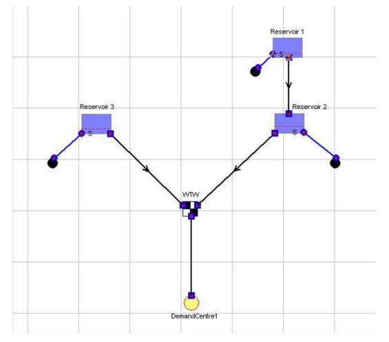
Figure 4 Example Aquator<sup>™</sup> schematic demonstrating a simple resource zone model with three reservoirs, a water treatment works, and a demand centre
