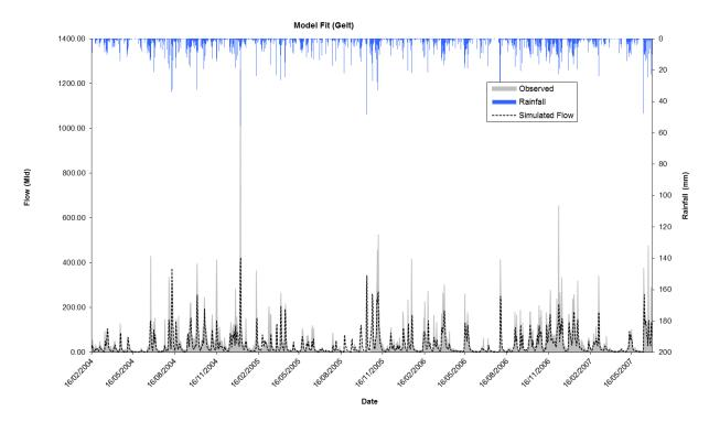
Figure 18 River Gelt (New Water) rainfall-runoff model fit, using parameters from the 2012 work
