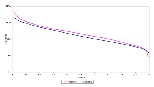
*Figure 19 Flow duration curve from the River Gelt (New Water) rainfall-runoff model, using parameters from the 2012 work*
