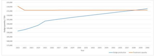
Note: The capacity line represents the treatment design capacity minus planned shutdown time.
