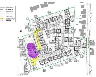
secured the discharge of all surface water to ground as opposed to our combined network. In line with industry standards for surface SuDS features, the basin was designed to store a 100 year event with an additional allowance for climate change. This provides a resilient alternative for surface water at this location.
